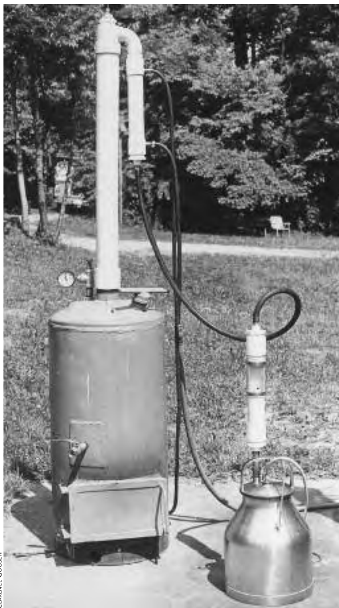
Fig. 8.32: A working demonstration model for vacuum distillation. Because of low operating temperatures, the column is fabricated from plastic pipe.
