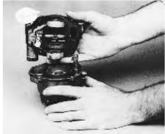
Fig. 9.8: Lifting the air horn to expose the float bowl.
