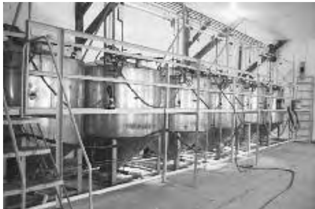
Fig. 4.1: A farm-scale ethanol fuel operation requires a commitment to time and equipment. These fermentation vats work on a continuous basis.
