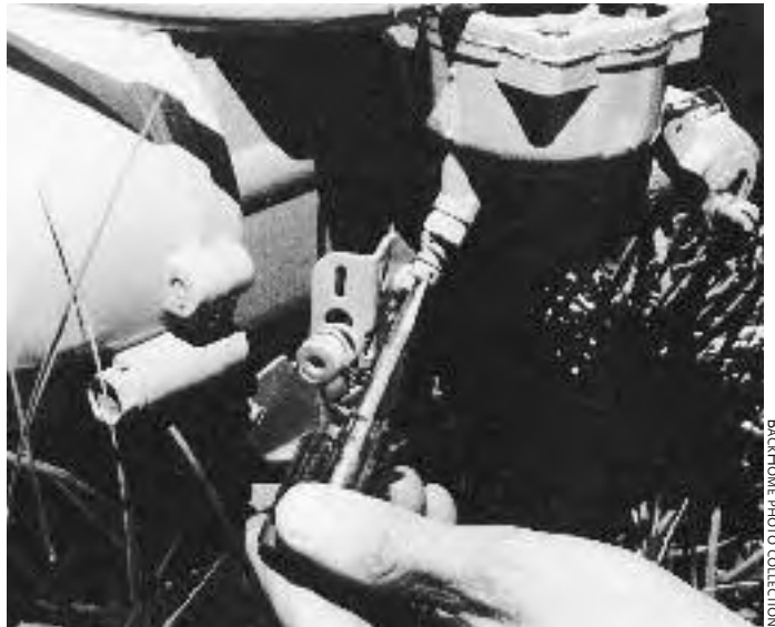
Fig. 9.25: Adjusting the main jet on a small four-stroke portable generator engine.
