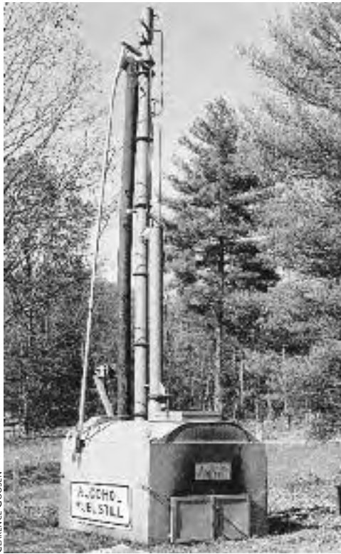
Fig. 8.4: A horizontal tank works well when used with a full-length firebox, built beneath the vessel. The flue at rear, behind the distillation column, allows combusted gasses to exit.
