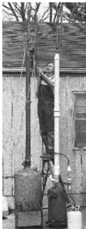
Fig. 8.13: Distillation columns used in commercial research for a major beverage distillery.
