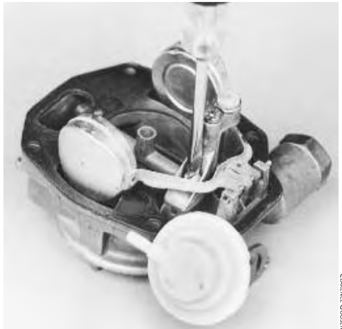
Fig. 9.9: Removing the jet tower.
