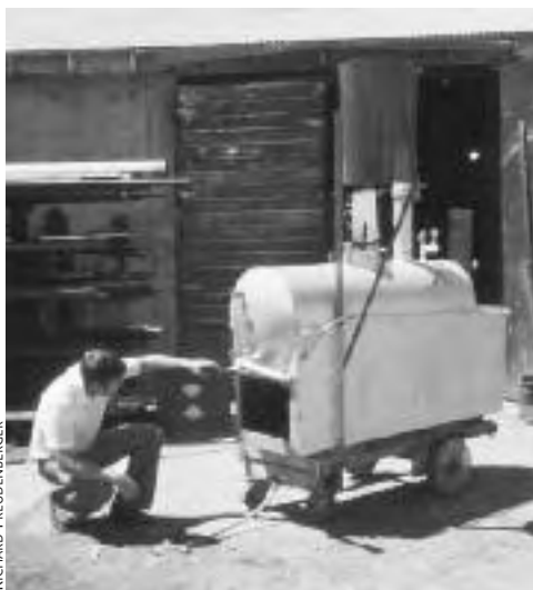
Fig. 3.5: Smaller distillation equipment can utilize wood fuel for heat very economically.
