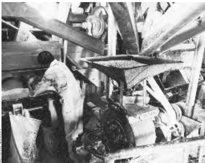
Fig. 6.2: A local mill or co-op can grind grains to the needed consistency for ethanol production.
