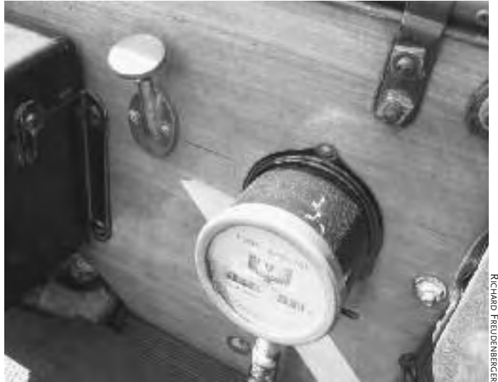
Fig. 1.7: The Model T Ford, manufactured through the 1920s, had a knob on the dashboard to control the setting of the carburetor’s main jet.
