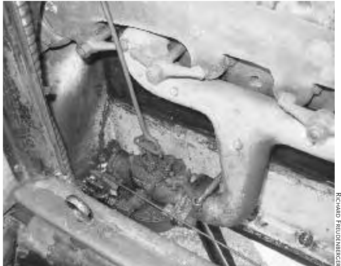
Fig. 1.8: The dashboard control knob is connected through a linkage to the carburetor so the engine can be adjusted to operate on fuel-grade ethanol.
