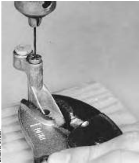
Fig. 9.10: Drilling the jet orifice with the proper size bit.
