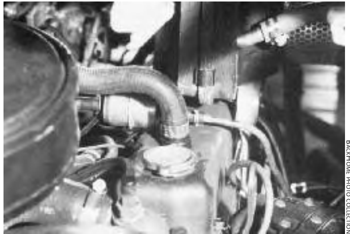
Fig. 9.23: The positive crankcase ventilation system (a portion of which is shown here, where the hose and valve is seated in the valve cover) provides a safe entry point for a spurt of gasoline used in cold starting.
