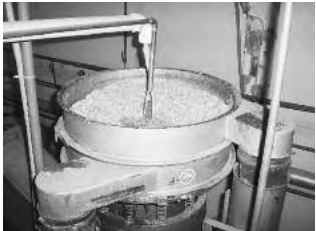
Fig. 10.3: Slurry is agitated to prepare mash for fermentation.
