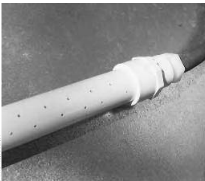
Fig. 6.4: An inexpensive and effective oxygen bubbling tube can be made from PVC plumbing parts.
