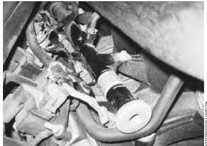
Fig. 9.18: Multi-port injection is more efficient than a TBI system, but is more costly because it requires more components. The fuel rail (dark tube, center) supplies the individual injectors, seen immediately to the left of the rail.
