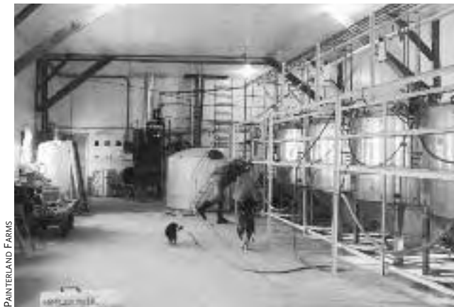
Fig. 10.5: The heating boiler and distillation column, seen in the back-ground. Fermentation tanks are on the right.
