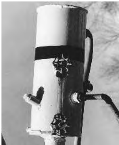
Fig. 8.18: The condenser at the top of a 6-inch column. The hoses are part of the cooling water circuit.
