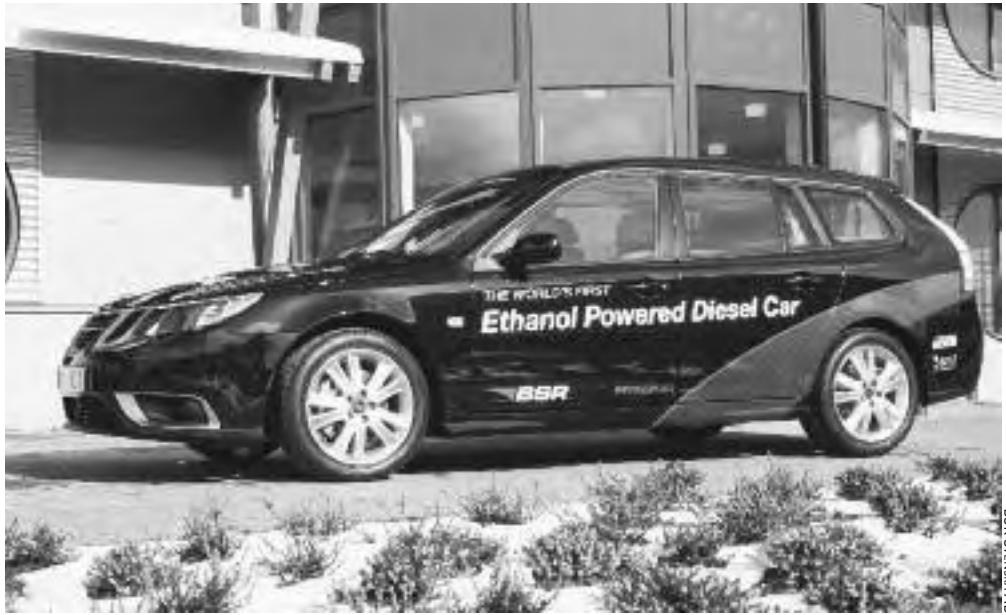
Fig. 9.28: The E-95 BSR Saab 9-3 utilizes ethanol in a diesel engine to reduce emissions by approximately 95 percent.
