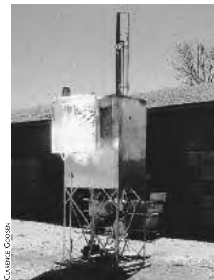
Fig. 7.11: Concentrated solar thermal energy being used to heat an oil medium for distillation in a 3-inch packed column, seen at rear.
