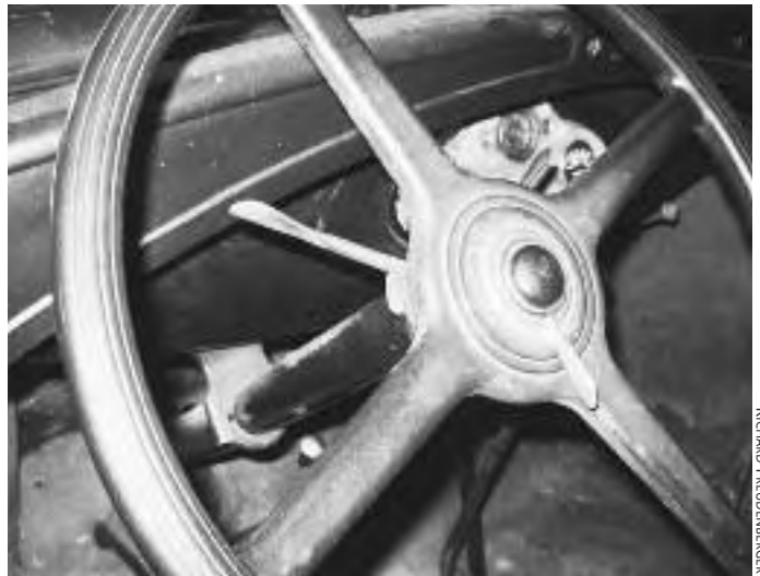
Fig. 9.20: In the early days of motoring, ignition timing was controlled manually by a lever, shown here on this 1930 Model A Ford.
