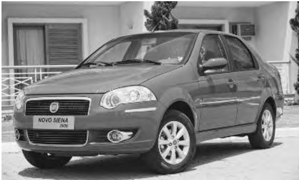
Fig. 1.15: The new Fiat Siena ELX 1.4 Tetraflex can operate on gasoline, alcohol, compressed natural gas or a combination of fuels
