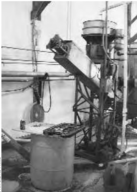
Fig. 8.2: An auger is used to transfer grain in this alcohol fuel plant at a Pennsylvania dairy farm.
