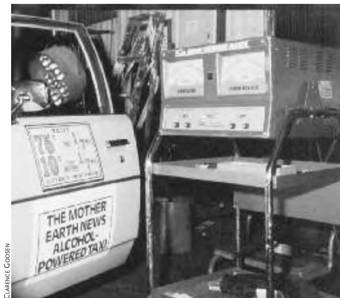
Fig. 9.2: Carbon Monoxide and Hydrocarbon emissions testing on a New York City taxicab for a press conference in June, 1979.
