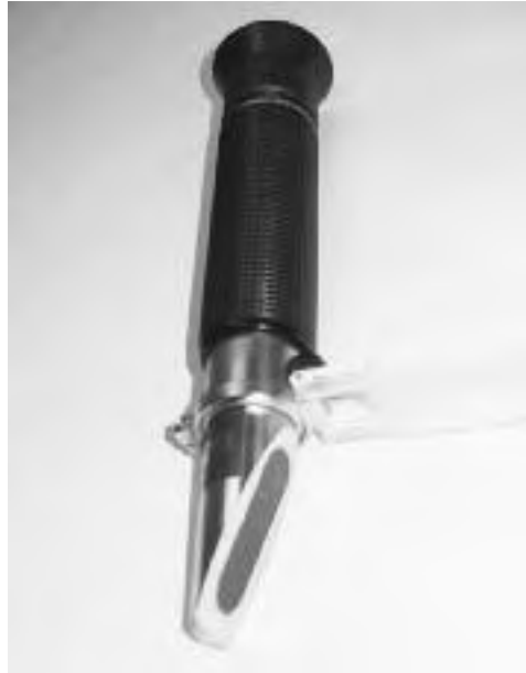
Fig. 6.12: A refractometer is used to give an accurate measure of sugar concentration in a potential feedstock.
