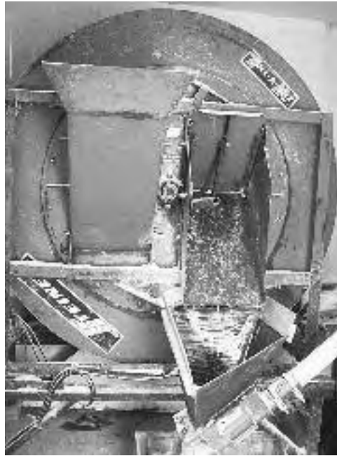
Fig. 10.2: A grinder/mixer includes a set of scales to weigh feedstock material.
