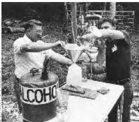
Fig. 8.29: Preparing to test proof strength of fuel alcohol from a small batch still.
