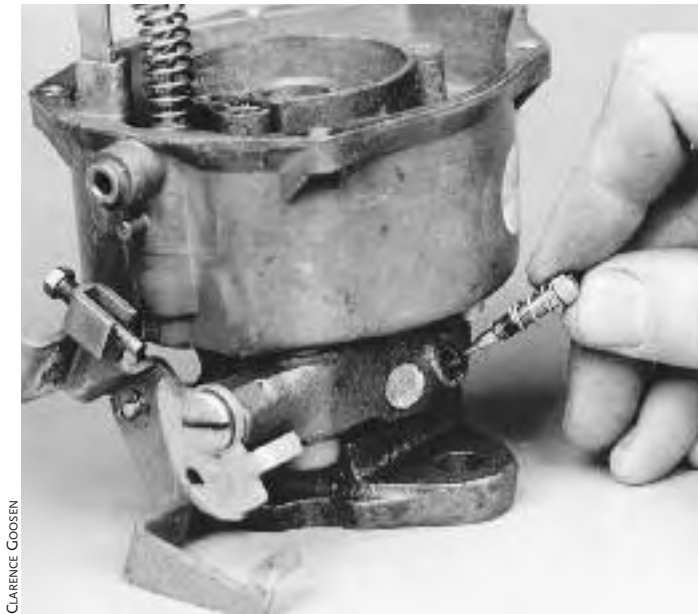
Fig. 9.13: Removing the idle screw exposes the orifice seat beneath it.
