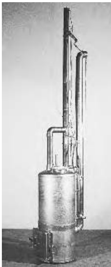
Fig. 8.15: A midpoint-entry column design, developed by Clarence Goosen, was used in several alcohol fuel distillation designs.
