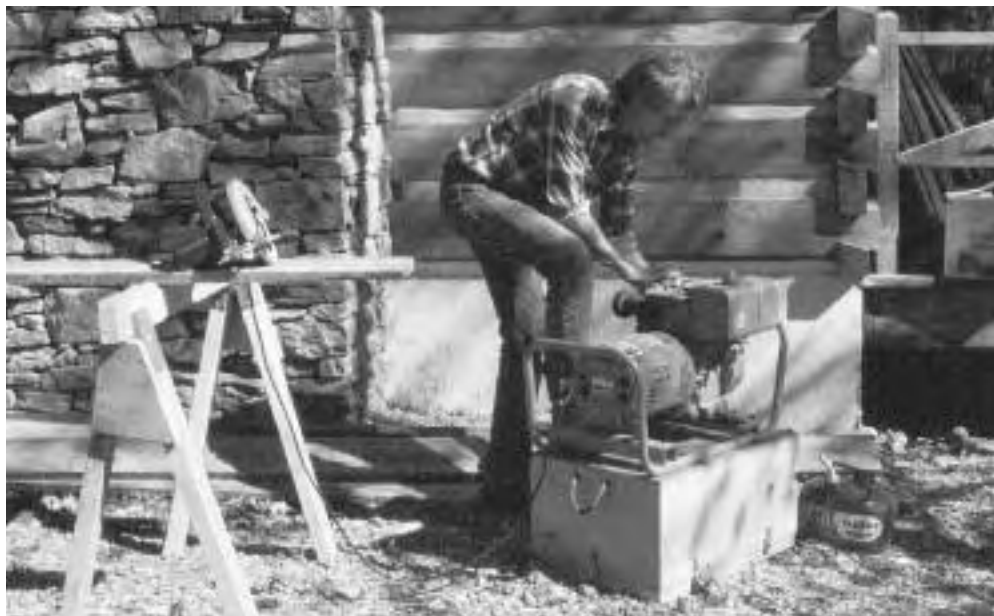
Fig. 7.9: The jobsite generator at this remote work site is fueled by hydrous 185-proof ethanol.
