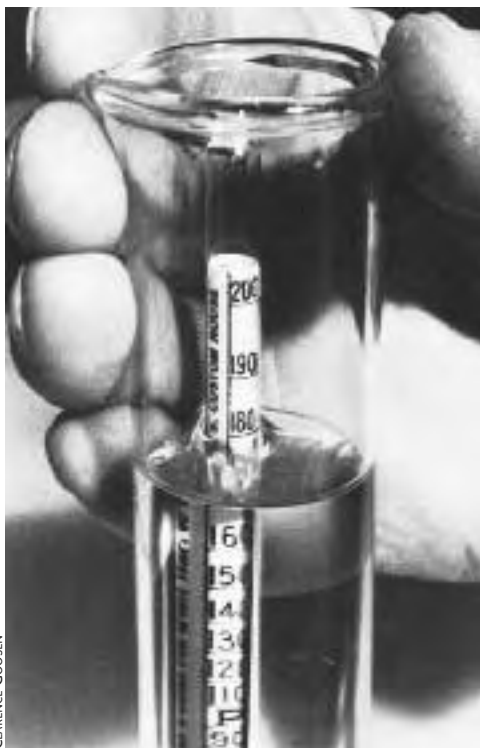
Fig. 6.13: A proof hydrometer measures alcohol content of a solution, when corrected to 60°F.
