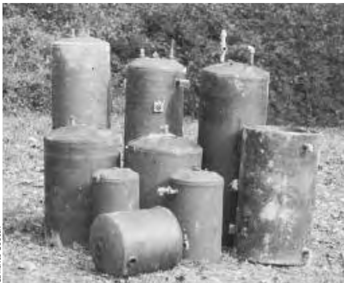
Fig. 4.2: Water tanks harvested from a scrapyard for repurposing as fermentation cookers and storage vats in a backyard operation.
