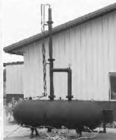
Fig. 5.3: Dan West's 6-inch packed- column still uses fruit waste and electric heating elements.
