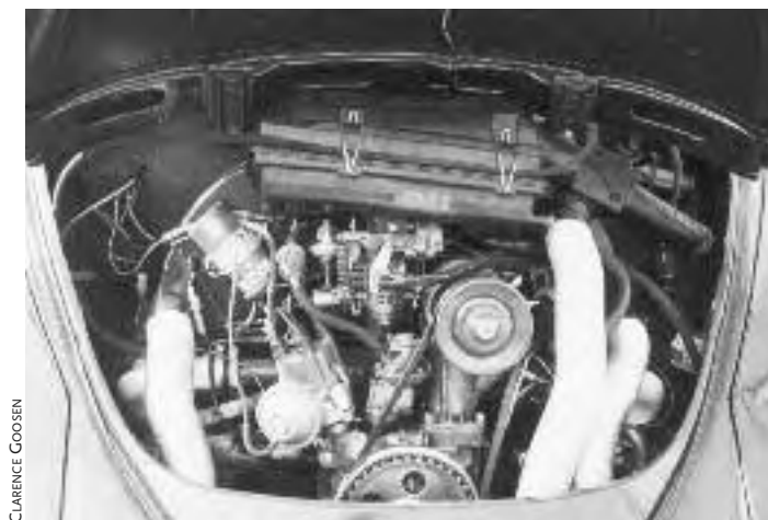
Fig. 9.1a: A tidy alcohol conversion on an older VW beetle uses air preheating as part of the technique.
