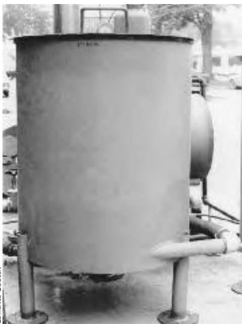
Fig. 8.8: A cooker vat for a 6-inch column still. Liquid mash is agitated and transferred through the pipe at bottom.
