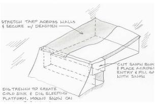
tapering the height of the walls, the tarp can be set on a slope to aid condensation run off during the night, and possible snow accumulation. It can also be constructed with a cold sink below the sleeping platform, and made large enough for several people, but it is not as warm as being completely surrounded by snow. Two people can construct a tarp roof shelter in 1 to 2 hours.
